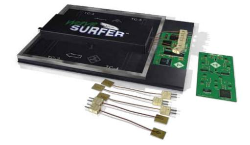
Check your wave soldering process and finetune your machine for optimum performance with the KIC Wave Surfer<sup>™</sup>.
